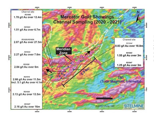
Figure 1. Geophysical map of the Meridian Zone showing the localization and gold assay values of selected channel samples
