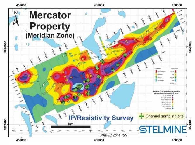
Figure 1. Contour map of the apparent chargeability determined by an IP/Resistivity survey completed on the Meridian Zone of the Mercator property. The IP axes and location of the channel sampling sites are reported on the map.
